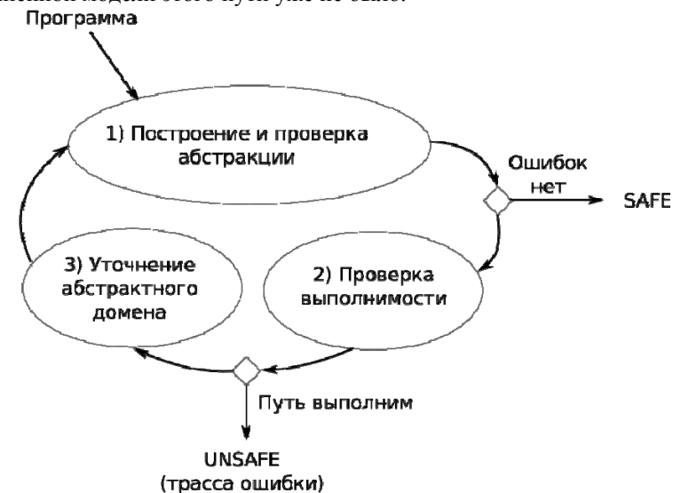
Рис. 1. Подход CEGAR (Counter Example Guided Abstraction Refinement)
