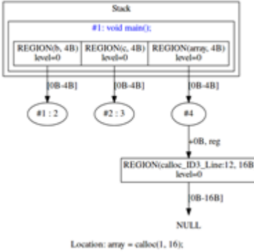
Fig. 4. Modification: allocate the 16 byte memory region on heap (mark it by tag calloc_ID3 ), fill it by NULL values, and assign to array a new point-to-value #4 which points to 0 offset of region calloc_ID3
