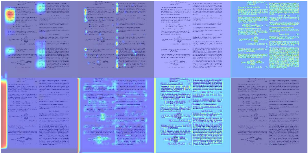
Fig. 10. The heat map obtained with GradCAM for the output layer of each of the four ResNet 18 blocks. Left is the conv_4, right is the conv_1. Bottom row contains heat maps for error model, Top row contains heat maps for fixed model. Trans+Ref image was used.
