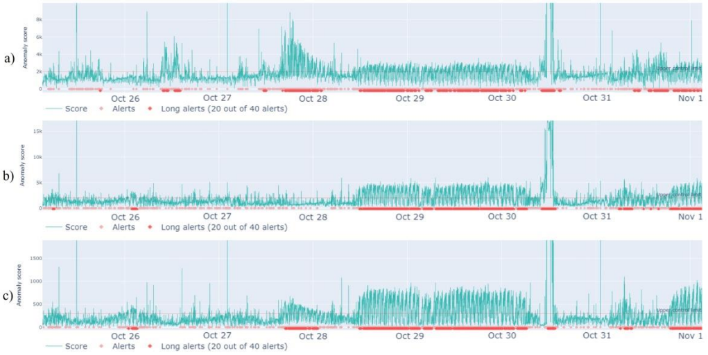
Fig. 13. Anomaly graphs for the 1st test period with TF-IDF weighting: a) logs only; b) tokens only; c) logs and tokens simultaneously.
