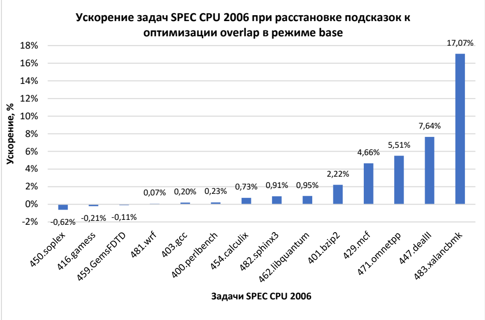
Рис. 7. Ускорение задач SPEC CPU2006 при расстановке подсказок к оптимизации overlap в режиме base. Fig. 7. Speed up of SPEC CPU 2006 benchmark with placement of hints to overlap optimization in base mode.
