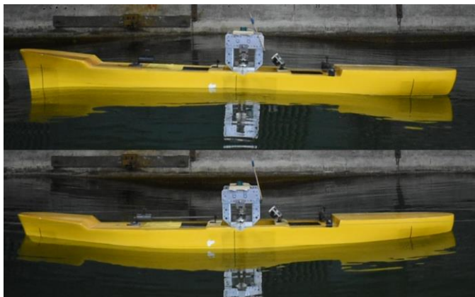
Fig. 7. Ship motions in head waves with a length of 4.0 m
