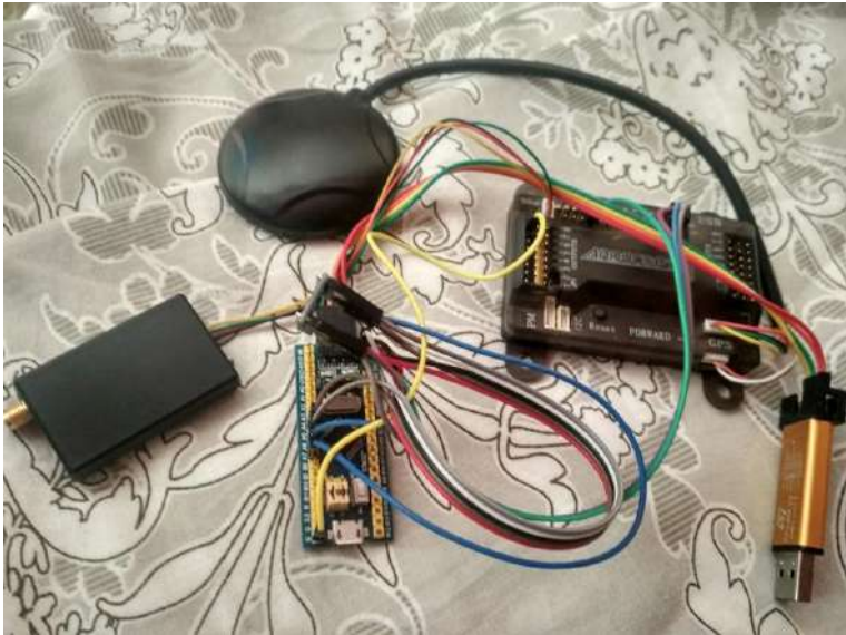
Fig. 16. Connection of the controllers using SPI bus
