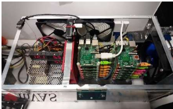
Fig. 1. Construction of Beowulf Cluster [9]
